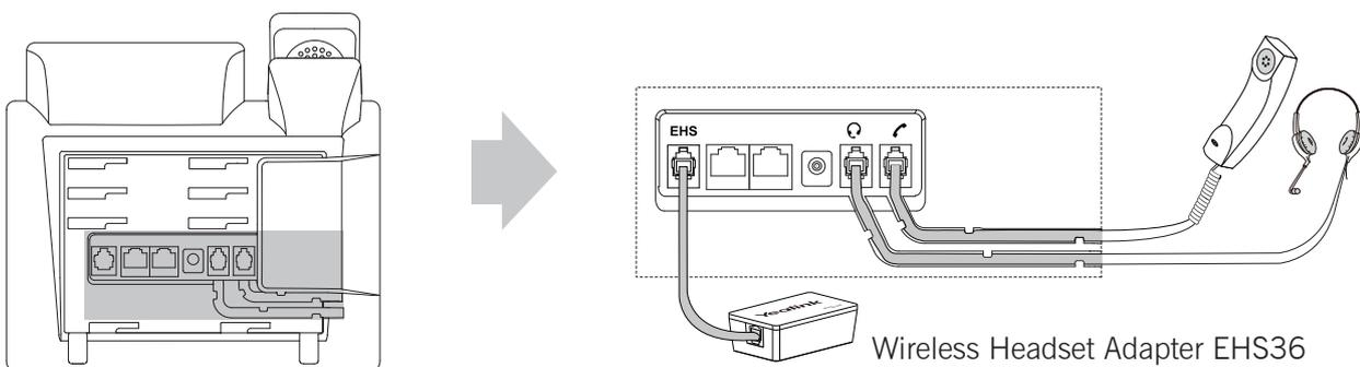
Note: The headset and wireless headset adapter EHS36 should be purchased separately. EHS36 is used for connecting the phone and a compatible wireless headset. For more information on how to use the EHS36, refer to Yealink EHS36 User Guide.
